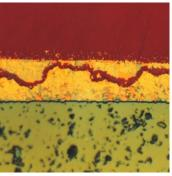
The use of active brazing alloys in a vacuum results in the direct wetting of oxide and non-oxide ceramics as well as the superhard materials cBN and diamonds. Besides joining, this process combination is also suitable for the metallization of ceramics and the application of functional structures onto ceramic substrates.
