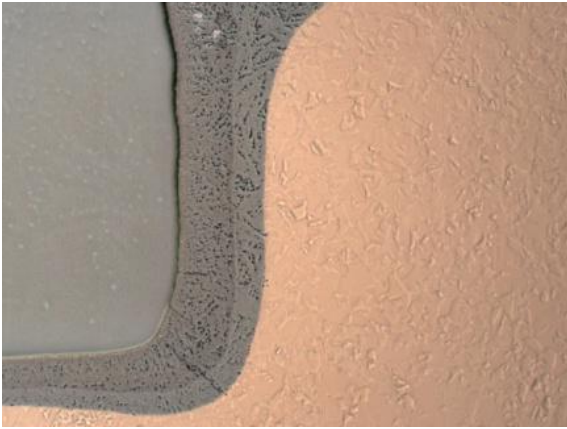
Fig. 1b: Joint Cu- to Ti-alloy, Pos. 4⇒5
