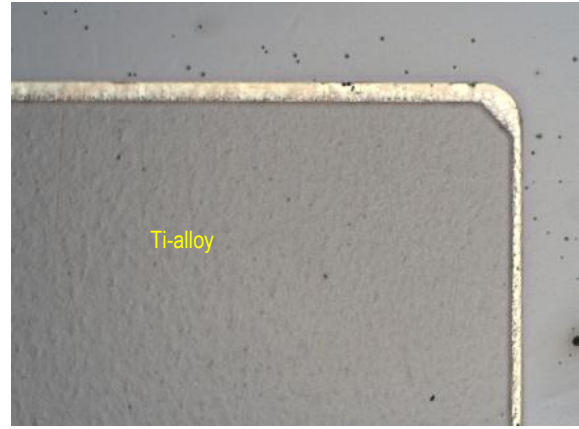
Fig. 2b: Joint steel to Ti-alloy, Pos. 2
