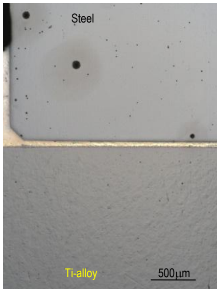
Fig. 2a: Joint steel to Ti-alloy, Pos. 1⇒2
